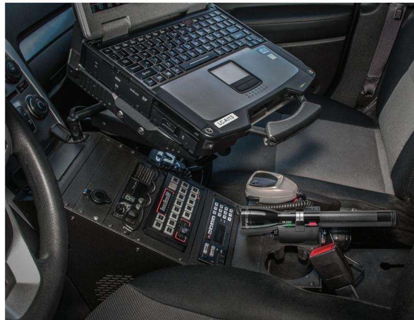
The cradle, mountable on any flat surface, has enough clamping force to secure the flashlight even when mounted upside down in a moving vehicle on a rough road.
