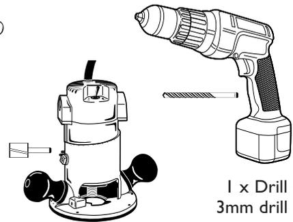
1 x Router + Ø26mm or less router bit
